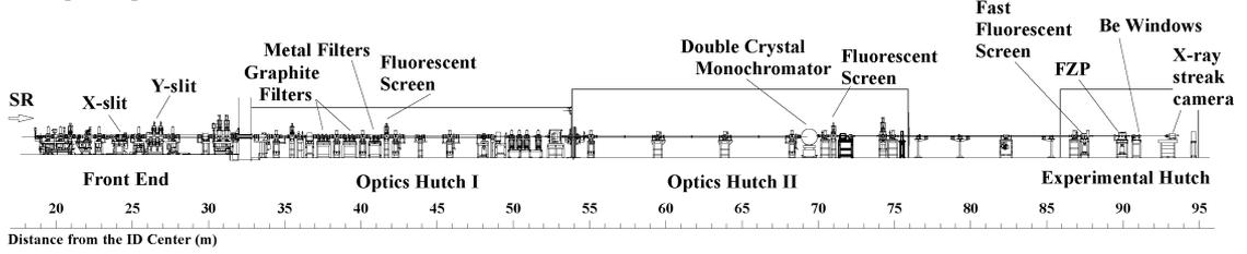
Figure 1: Schematic view of the SPring-8 diagnostics beamline II (BL05SS).
