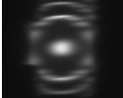
Figure 4: Observed angular spectral flux at the photon energy of 8.3 keV corresponding to the peak of the 19th harmonic for the minimum magnet gap of 20 mm. The center spot is the 19th harmonic radiation, and two outer rings correspond to the off-axis radiations of the 20th and 21st harmonics.
