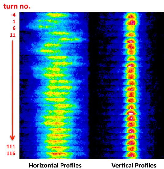
Figure 6: An example of the profiles of the photon beam of the ID obtained every 5 turns by the TTPM. The left and right images are for horizontal and vertical profiles, respectively. The numbers on the left side show the turn numbers after injection for topping-up of which the turn of the bump orbit excitation is labeled as the zeroth turn (see text).
