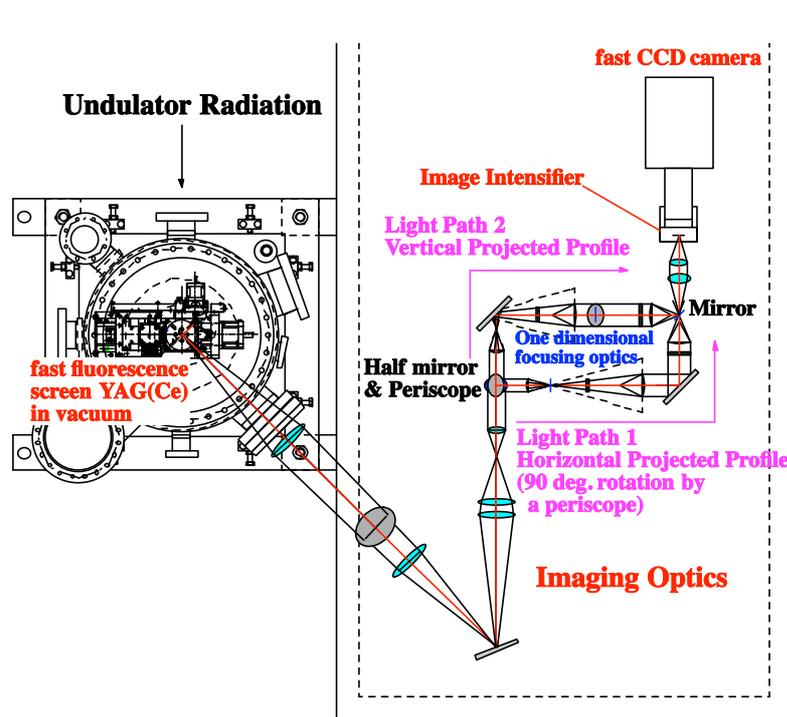
Figure 5: Experimental setup of the turn-by-turn beam profile monitor (TTPM) developed at the diagnostics beamline II (BL05SS).
