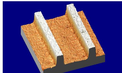
AFM measured groove shapes
