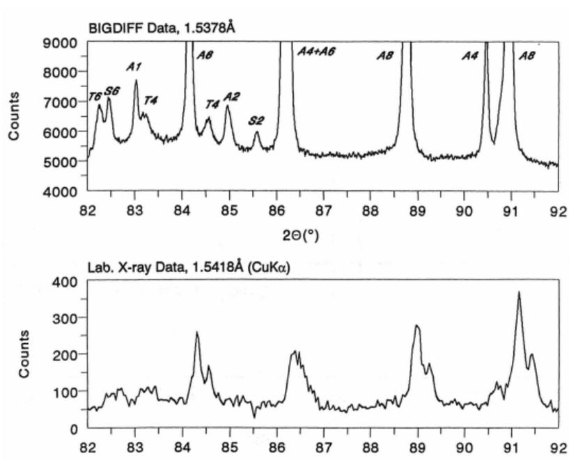
Multi-phase ceramic:  $\alpha$   $\text{Al}_2\text{O}_3$ ,  $\text{ZrO}_2$ ,  $\text{MgO-Al}_2\text{O}_3$  (spinel).
