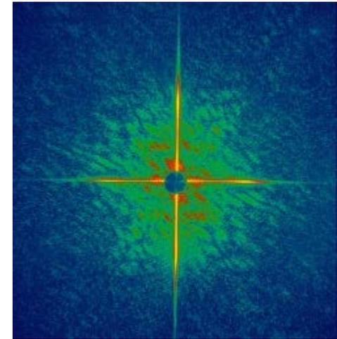
A coherent diffraction pattern of the object recorded from a single 25-femtosecond FEL pulse.
