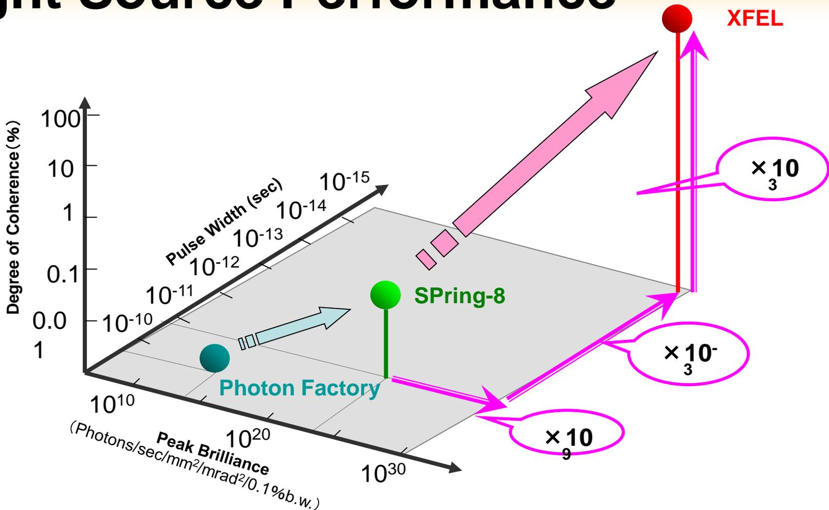
**Remarkable Features of XFEL producing  $\lambda < 0.1$  nm X-Rays**
