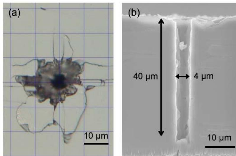
Fig. 2. (a) Optical microscope image of irradiated silicon viewed from surface at fluence of  $57 \mu\text{J}/\mu\text{m}^2$ . (b) Cross sectional SEM image of (a) prepared by focused ion beam sampling.
